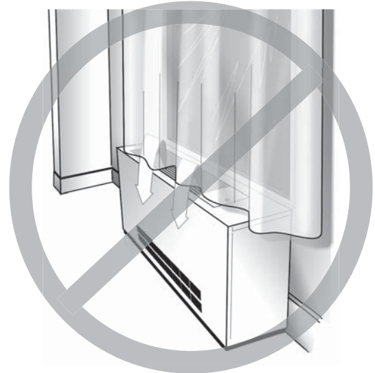
Figure 7 Restricted air flow diagram
