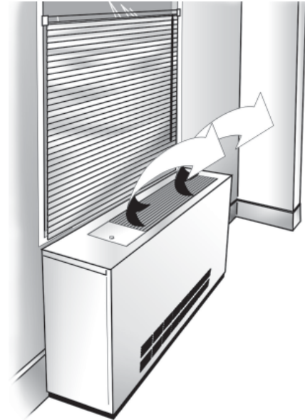
Figure 6 Proper air flow diagram
