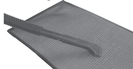
Figure 29 Cleaning With A Vacuum
