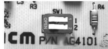
DIPSWITCH ON RELAY BOARD
