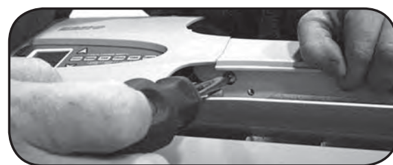
Figure 8 Lift front grill to expose screw
