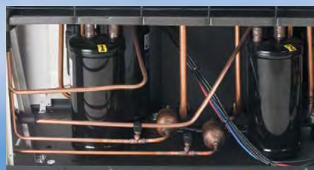
Independent Refrigerant Circuits
